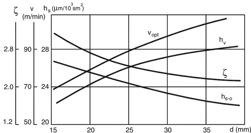
**Fig. 7** Influence of the diameter of the hole being machined on  $h_{s-o}$ ,  $v_{opt}$ ,  $v_{ho}$ , and  $\zeta$  at the invariable optimal cutting temperature. Turning, work material: stainless steel AISI 303, tool material: carbide M20 (92%WC, 8%Co)
