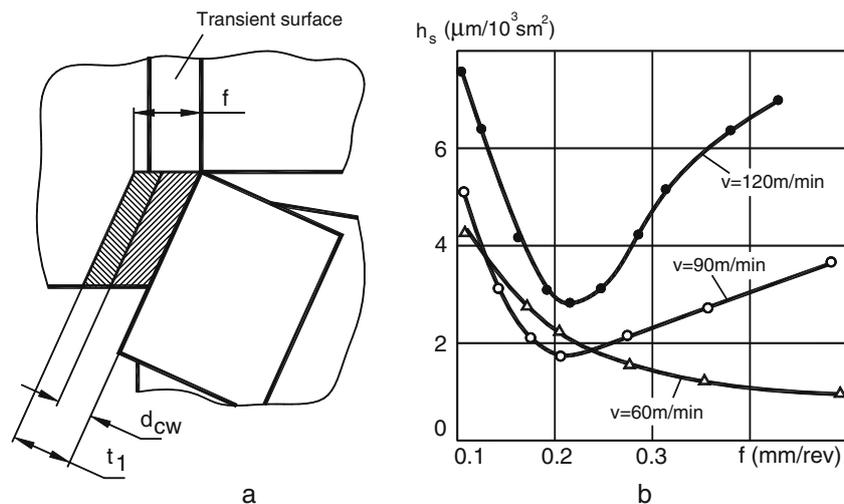
**Fig. 2a, b** Illustration of the depth of cold working of the transient surface (a) and influence of the feed on the tool wear rate (b), work material: stainless steel AISI 303, tool material: carbide M10 (97%WC, 3%Co), depth of cut  $d_w=0.5$  mm
