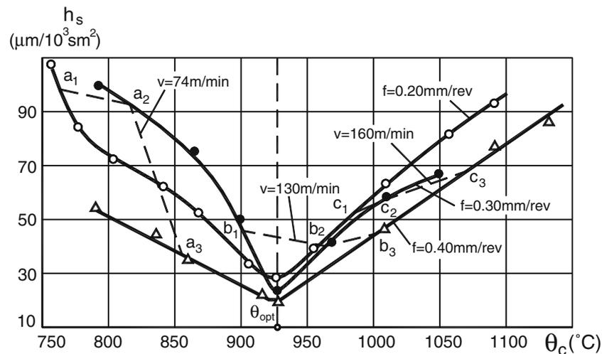
**Fig. 1** Influence of the cutting temperature on the relative surface tool wear rate in turning AL 610 alloy, tool material: carbide P10 (14%TiC, 8% Co), depth of cut  $d_w=1$  mm
