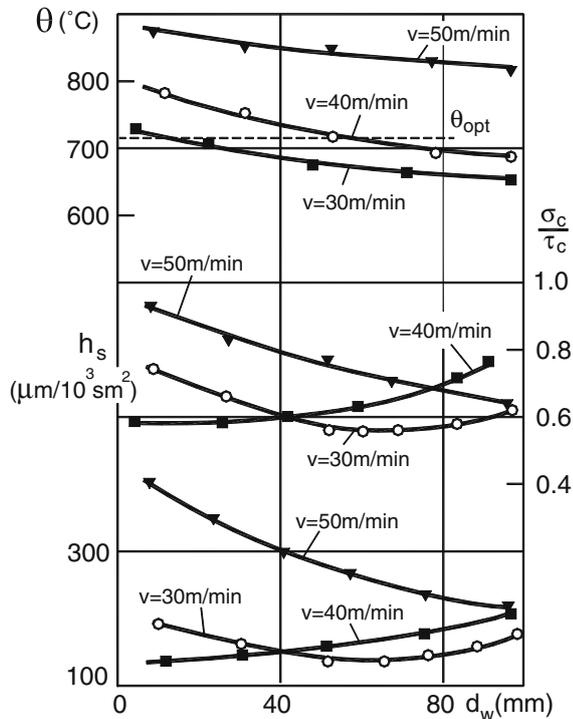
**Fig. 5** Influence of the cutting speed and diameter of the workpiece on the cutting temperature, contact stress ratio at the tool–workpiece interface, and optimal tool wear rate in turning, work material: Haynes 263 alloy (29%Cr, 2.5%Ti), tool material: micrograin carbide M10 (94% WC, 6%Co), depth of cut  $d_w=0.25$  mm, cutting feed  $f=0.09$  mm/rev
