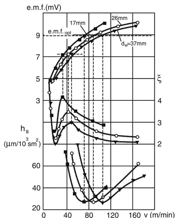
**Fig. 6** Influence of the cutting speed and diameter of the hole being machined on the cutting temperature and the tool wear rate, work material: stainless steel AISI 303, tool material: carbide M20 (92% WC, 8%Co), depth of cut  $d_w=0.30$  mm, cutting feed  $f=0.06$  mm/rev
